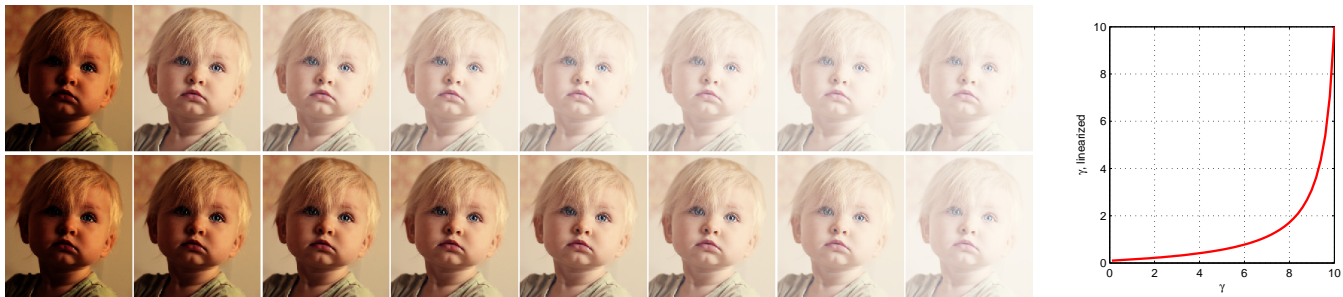
Figure 1: Example linearization, for demonstration purpose, using a simple gamma mapping value as parameter, I_p = I^{\frac{1}{p}} . Left: Output with equal sized steps of gamma (top) and after linearization (bottom). Right: The transformation function, \hat{f}^{-1}(p) .
