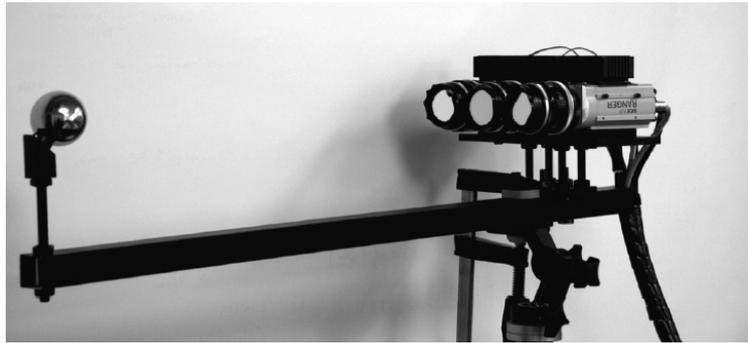
**Figure 3:** The single lens setup with an RGB beamsplitter (left), and the simpler setup with three separate lenses and RGB color filters pointing at a reflective sphere (right). Both use three separate, unmodified but reprogrammed C55 camera units.
